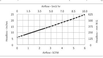
Above curves are generated based on ideal condition. Actual curves for specified project/condition to be provided upon request.
